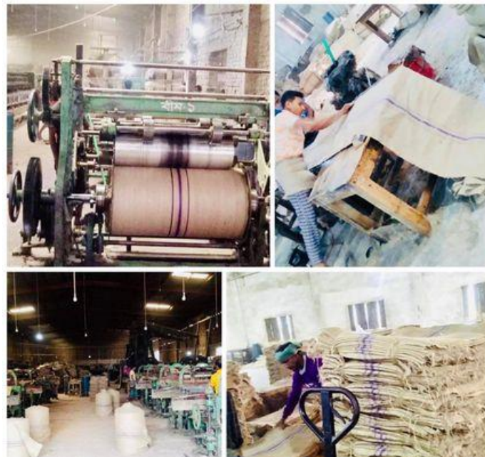
Figure-16: The Manufacturing Process of Jute Bags
