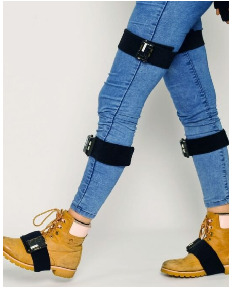
Figure 2.9: Use of IMU sensors to analyze gait patterns [2].
