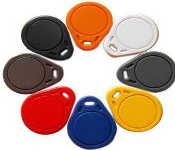
Figure 2. 7 : Passive tags of RFID
