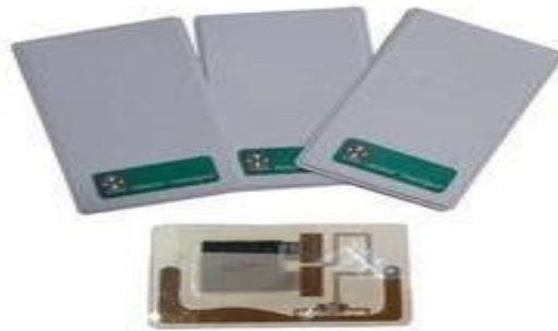
Figure 2. 8: Semi passive tag of RFID
