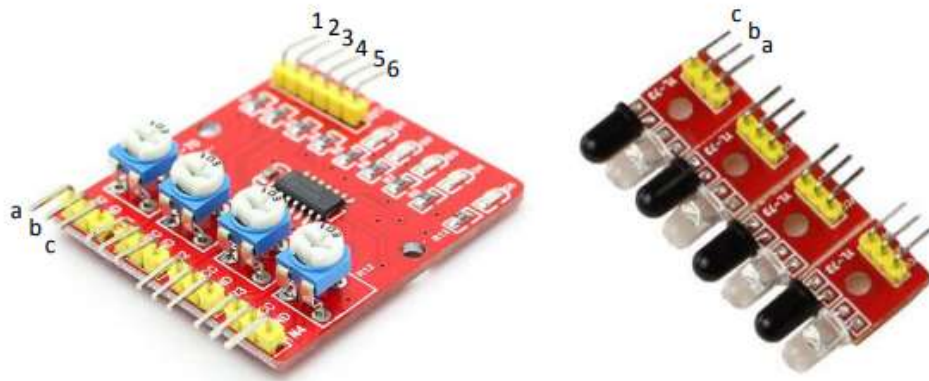
Figure 2. 15: IR sensor (4-Way IR Infrared Tracking Sensor Module)
