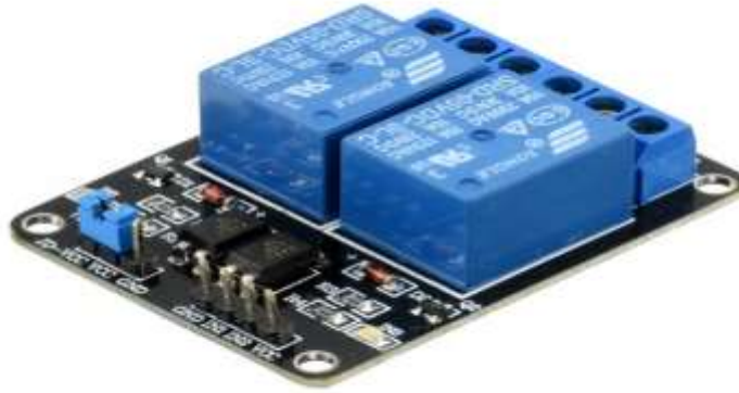
Figure 2. 17: 2-Way Relay Module
