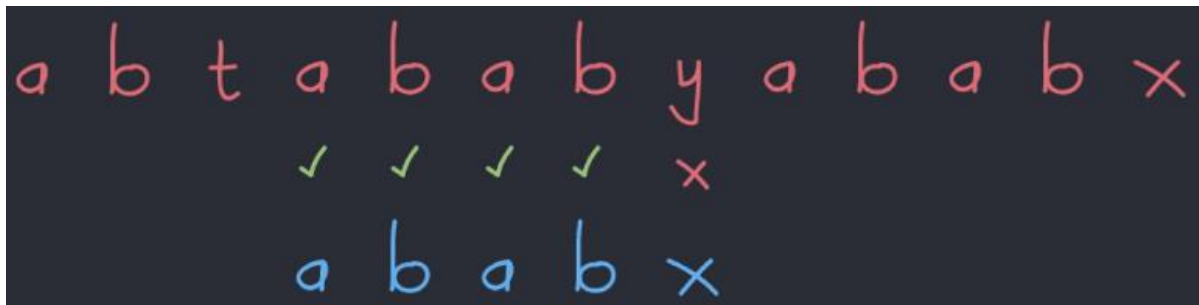
Figure -3.3.3: In this iteration, we are seeing that the text character “y” is not matching with the pattern character “x”. So from the failure function, we can see that we have to move the second “a” pattern character into the text character “y” index.
