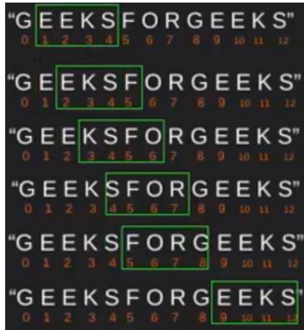
Figure -3.2.2: The text window will shift like this and the length of the window will be the same as the length of the pattern size. Based on this window length, every hash value will be generated for each window, and after that, the hash value and every window hash value of the text will be compared.
