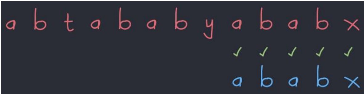
Figure -3.3.6: Here we can see that all the character of the pattern and text is matching so we can say we have a match found!
