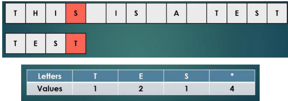
Figure 3.5.9: In the first iteration here we can see pattern character “T” is not matching with the text character “S”. According to bad match table, we can see we have to forward 1 index. So we will slide the pattern 1 index right and again try to match pattern with the text from rightmost.
