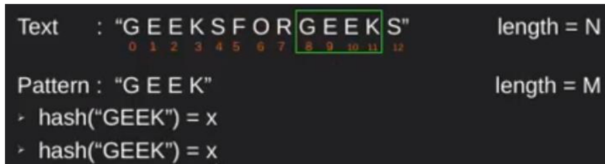
Figure -3.2.11: In this iteration, the hash value of the pattern is matching with the hash value of the sub-string of the text. Because of it is matching now algorithm will try to match character by character and all the characters are matching so algorithm will say the pattern is found in the index 8. After that, it will shift the window right once.
