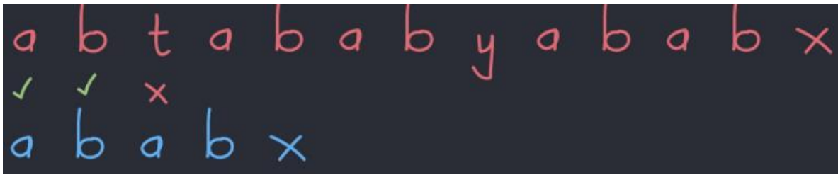
Figure -3.3.2: At the very beginning iteration we are seeing that text character “t” is not matching with the pattern character “a”. the last match shows us that we have to shift the whole pattern into the text index where “t” is located.
