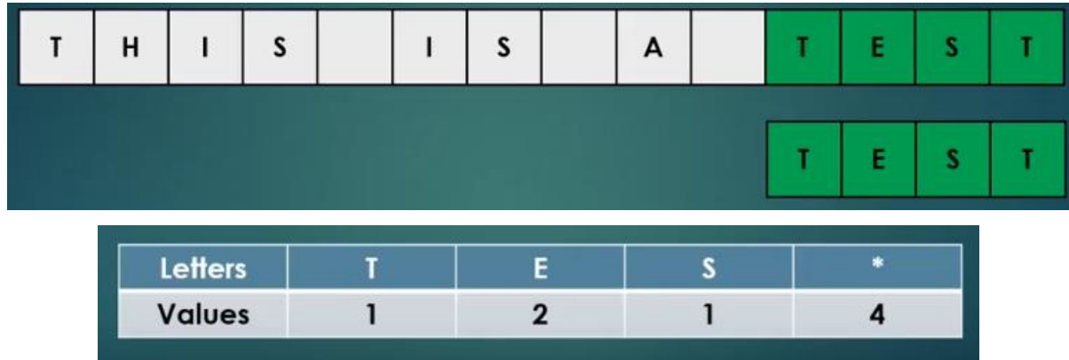
Figure 3.5.13: Here we can see pattern character “T” is matching with the text character “T” and after that, all the characters of the pattern is matching with the characters of the text. So we found a match!
