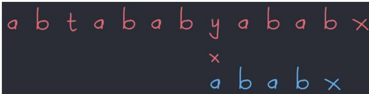
Figure -3.3.5: In this iteration, we are seeing that the text character “y” is not matching with the pattern character “a”. Because the first thing is mismatched so we have to shift one index.
